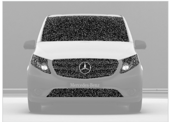
Front of vehicle - speckled areas: Areas where wrapping is not permissible (example Metris cargo van, schematic diagram)
