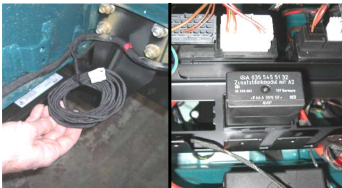
CODE L77 - Wiring for additional turn signals left/right, wire located at rear cross member, blink module located in driver seat pedestal
