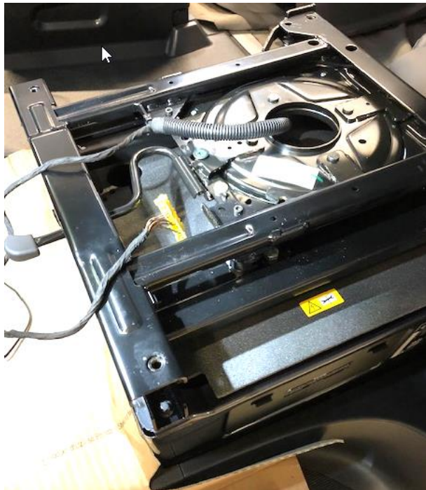
Driver swivel seat base with seat harness unsecured (yellow connector).
