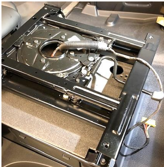
Passenger swivel seat base with seat harness unsecured (yellow connector).
